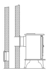
Rear flue connection into chimney with sealing collar. Cleaning door on opposite side
