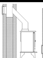
Top outlet with 45 degree bend sealed into masonry chimney with cleaning door on opposite side.
