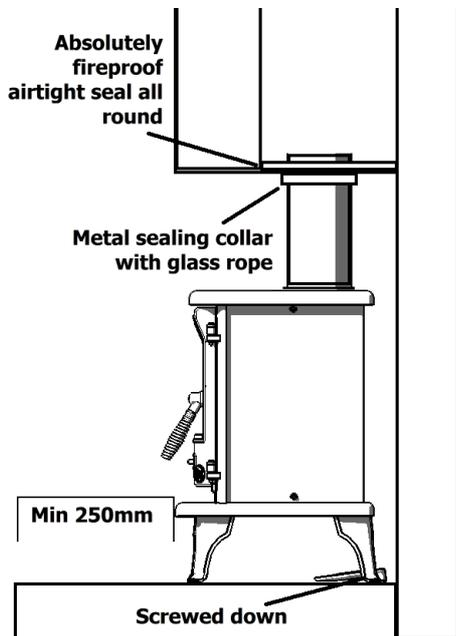
Typical installation in masonry fireplace with solid hearth extending at least 250mm in front of stove. Completely and absolutely sealed into oversize chimney.
