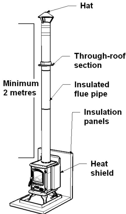
Where the stove is to be fitted in a shed, inland marine craft or other building for occasional use a 100mm internal diameter flue may be used, with the proviso that the flue is:
