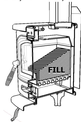
Place two or three firelighters close together, or screwed-up paper covered with dry sticks, at the back of the grate and light them. When they are burning well gently fill the fire with dry fuel, close the door and set the air control slide to the 'high' (right) position. When the fire is burning well, move the control to the lowest practical setting.
