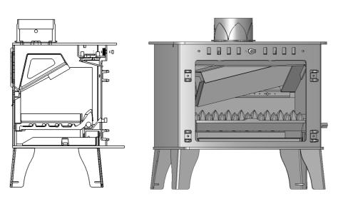
Lift the Baffle and slide to the left.
