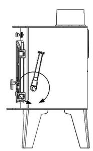
**To burn wood**, push the operating tool up and away from you. When left in this position, air is restricted through the bed of the fire providing a solid base to build up a bed of ash. Surplus ash can be removed either by gentle riddling or with a shovel.
