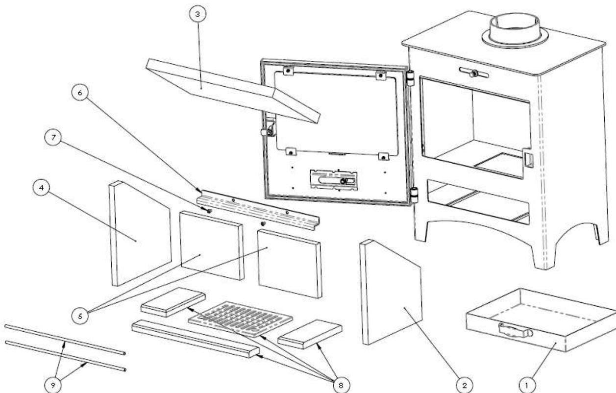
To install the internals simply follow the numbered sequence 1-9 and to remove simply reverse this process.
