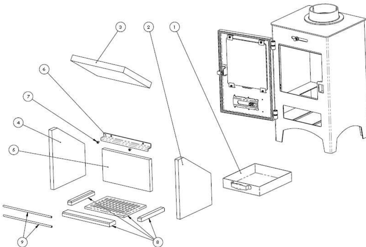
To install the internals simply follow the numbered sequence 1-9 and to remove simply reverse this process.
