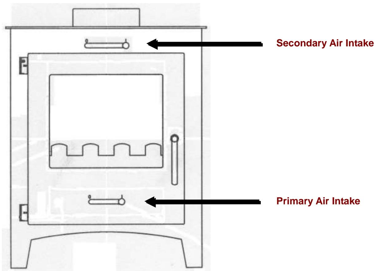
The main door handle on these appliances will get hot but are removable. To remove the handle, simply lift the main handle upwards between periods of refuelling.
