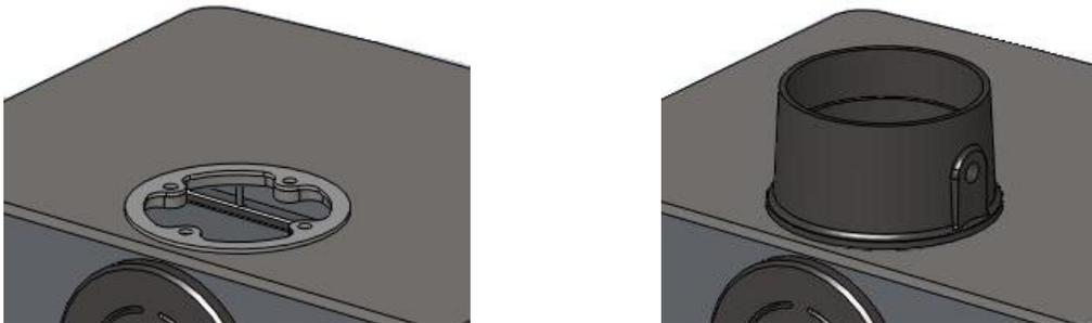
Place the Flue Gasket on the top, or rear outlet as required. Place the Flue Collar on top of the Gasket. Secure to the four locating tabs, inside the flue outlet, using the M6 screws supplied. Fit the 2 - M8 carriage bolts, washers & nuts into the Damper Holes, located on each side of the Flue Collar.
